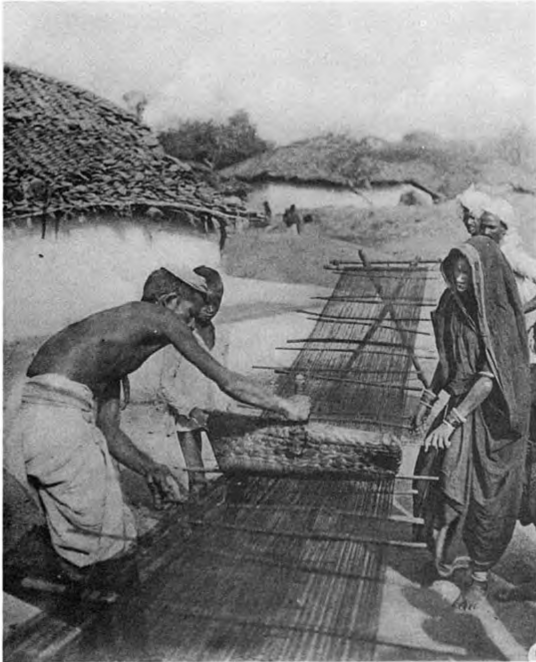
Weaving: sizing the warp
